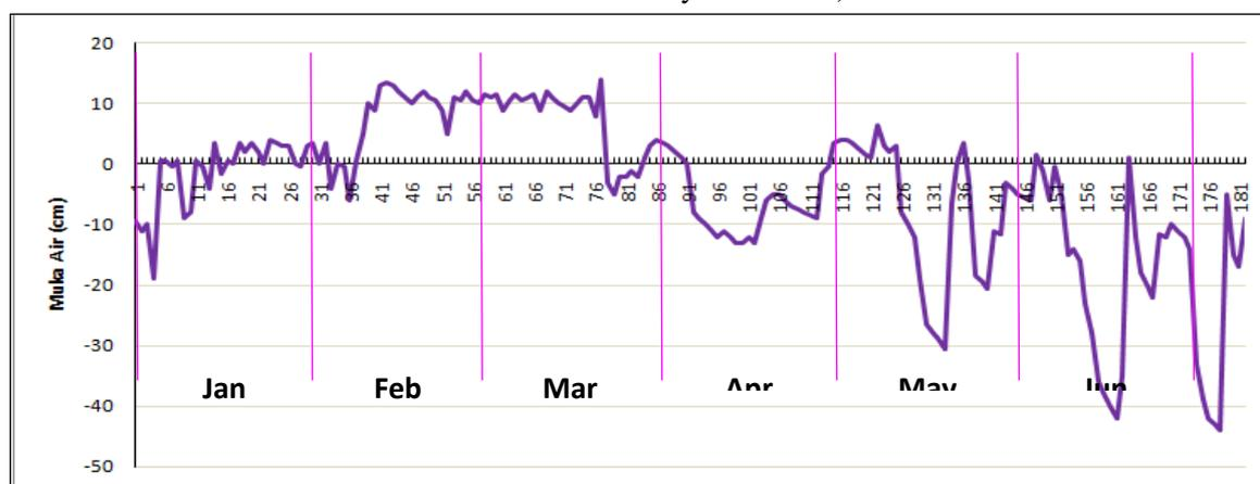
Figure 6. The Effect of TC4 water retention on Water table fluctuation within the soil at the observation Well 5
