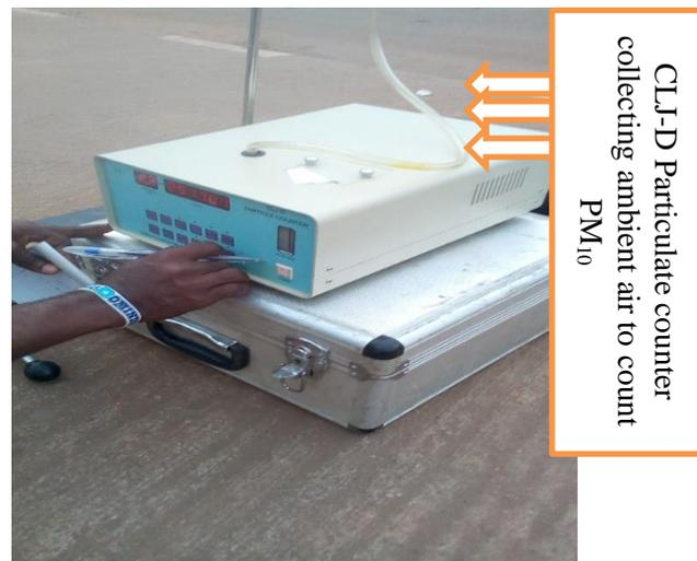
Figure 4. A CLJ-D Particulate counter in use on the field
