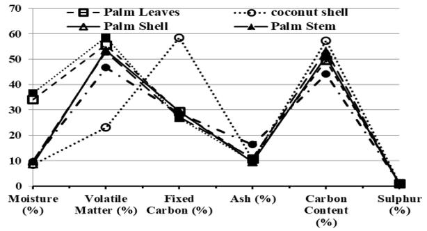
Figure 3. Graph of bio-coal chemical composition based on biomass type
