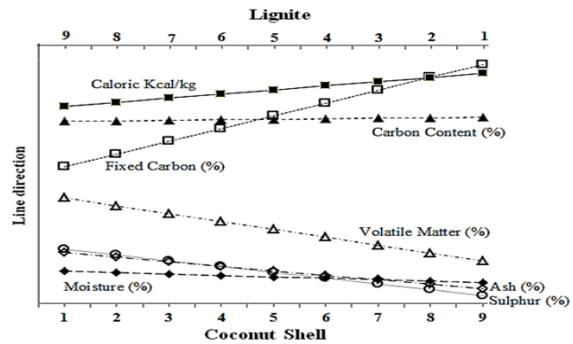
Figure 4. Line direction based on the composition of coconut shell to lignite in wt %
