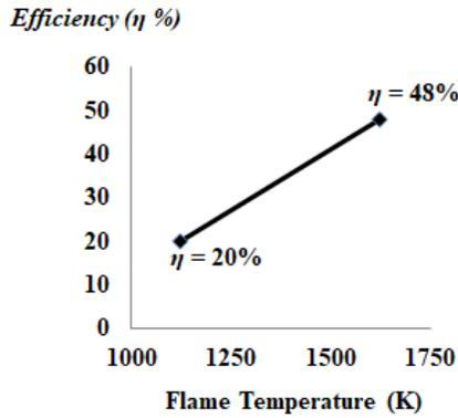
Figure 1. Relationship between flame temperature (K) and furnace efficiency.  $\eta = 20\%$  and  $\eta = 48\%$
