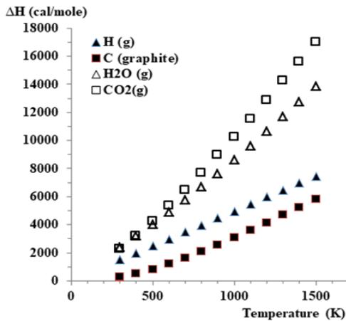
Figure 2. The relationship between the combustion reaction temperature (K) and enthalpy (cal/mol)
