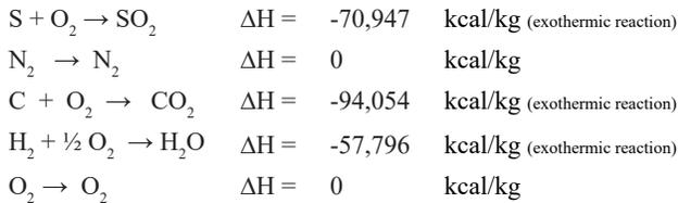
The amount of chemical content above in the fuel will result in greater enthalpy differences. The higher the combustion temperature the larger the resulting enthalpy. The relationship between
